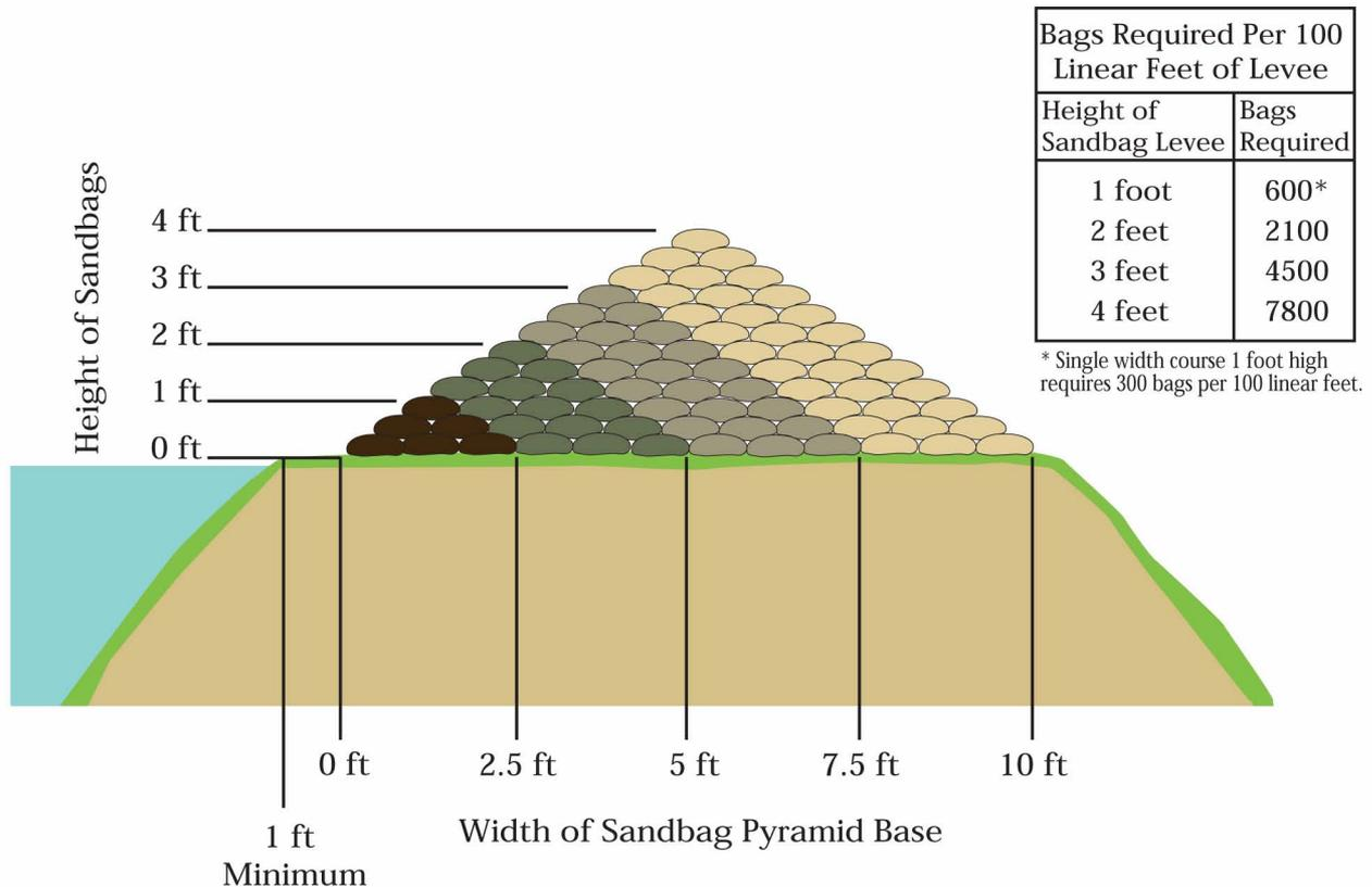
The pyramid placement method is used to increase the height of sandbag protection.
